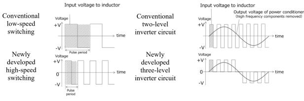
Fig. 3 Switching of power semiconductor devices
